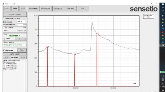
Figure 3: Sensetio Pro – GSR and HRV - mouse measurement system. Indices T1–T3 are identified significant events during the measuring. (Source: Authors).
