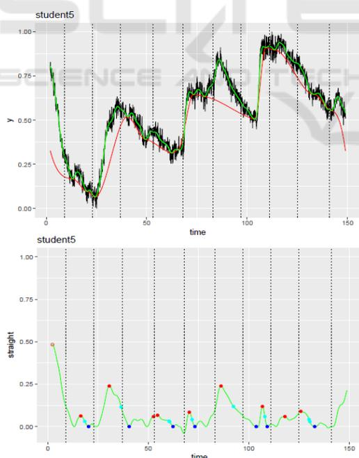
Figure 4: Sensetio Pro analyzer analyzes raw data, interleaves them with a baseline curve (graph above), converts raw data into filtered smoothed data, where peaks, false peaks, monotonic intervals, etc. are identified (graph below). (Source: Authors).
