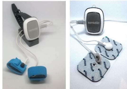
Figure 2: Bluetooth GSR measuring system – a wristband with finger contacts (left picture), wristband with adhesive back contacts (right picture).
