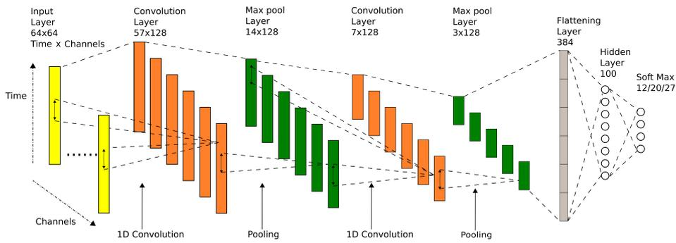
Figure 3: Flowchart of the multi-channel CNN for multivariate time-series modeling.
