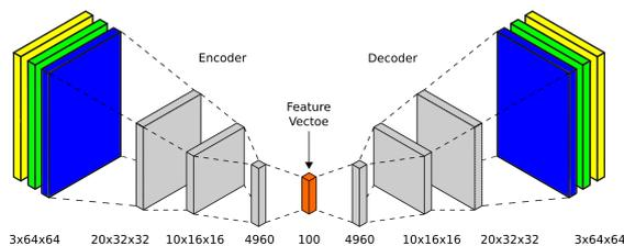
Figure 1: Architecture of convolutional autoencoder.
