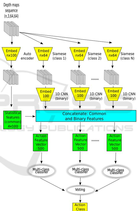
Figure 4: Ensemble operating on features extracted by convolutional autoencoder, concatenated with class-specific features that were extracted by Siamese neural networks.
