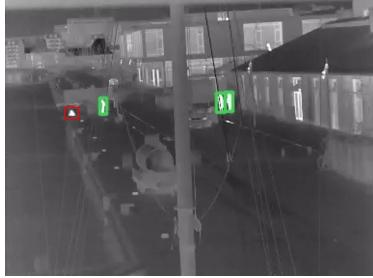
Figure 7: A failed case which should have raised an alarm. The red box refers to the undetected person.
