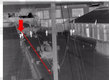
Figure 1: Thermal surveillance imaging for detecting potentially dangerous situations and alerting authorities. An alert should be raised when someone crosses the red line.
