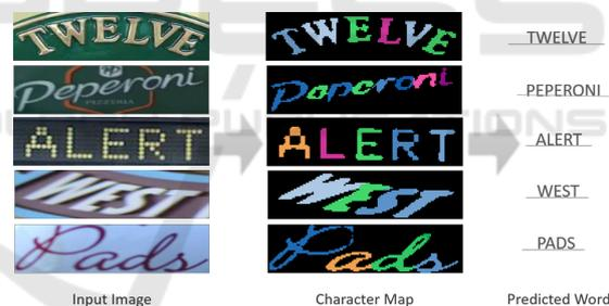
Figure 1: Examples taken from irregular text datasets, which include rotated, curved, distorted, and multi-font text. Our model first outputs a character map, then the map is used to generate a word.
