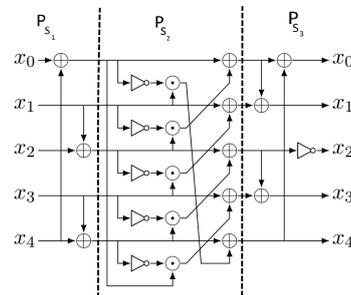
Figure 4: Binary network for the S-box in  $p_S$  permutation divided into  $p_{S_1}$ ,  $p_{S_2}$ , and  $p_{S_3}$ .
