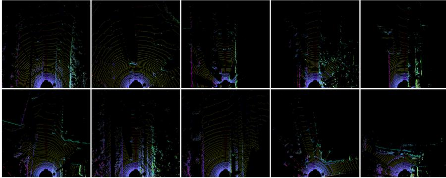
Figure 3: **The Visualization of Normal-map.** A 2D BEV feature map based pseudo-image contains the 1st-order features (surface normal) of objects.
