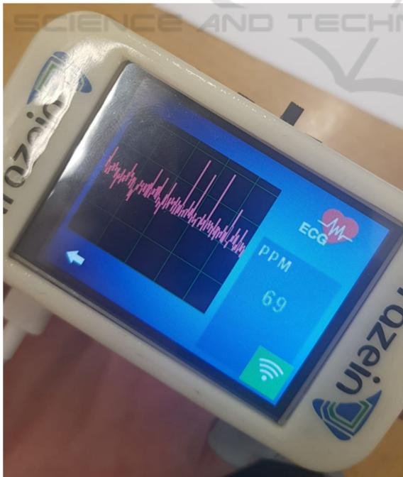
Figure 7: Trazein HMI showing ECG signal and BPM real-time acquisition with one subject.
