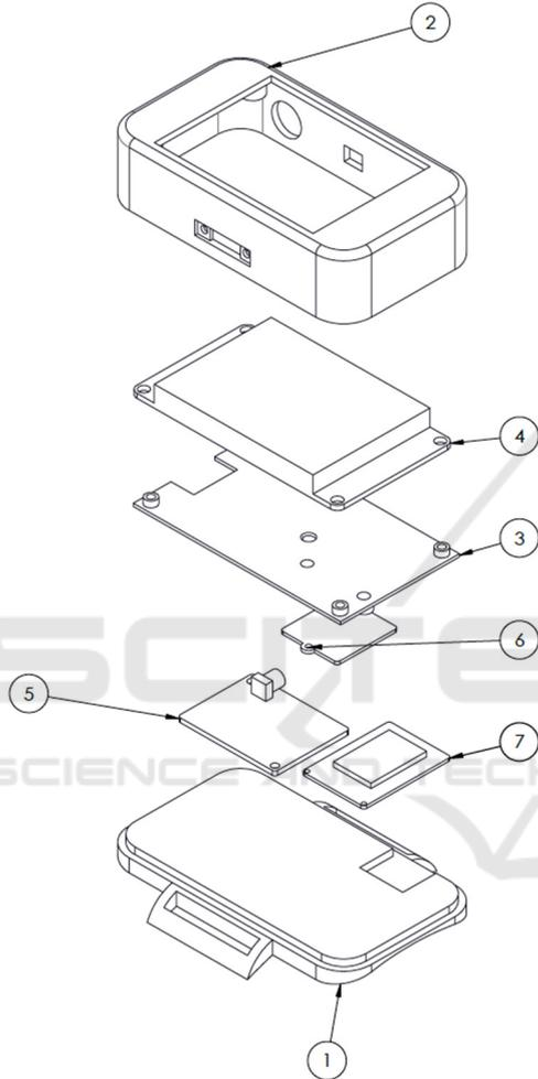
Figure 1: Exploded Device with Fusion360 CAD Software. “Fit to wrist” configuration.
