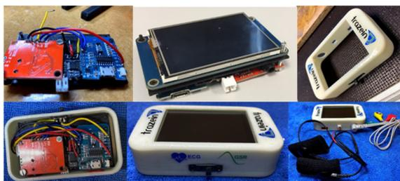
Figure 5: Final 3D printed manufactured device.
