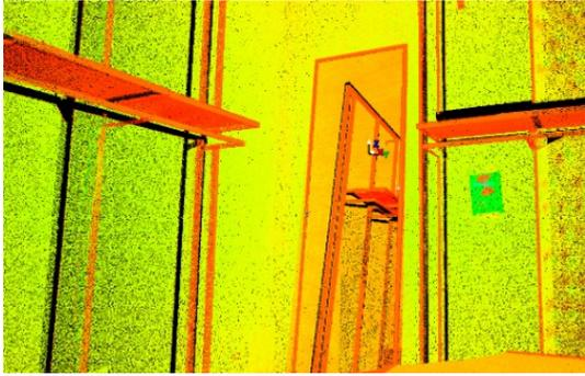
Figure 1: Laser scanning next to a mirror at a department store (point cloud).
