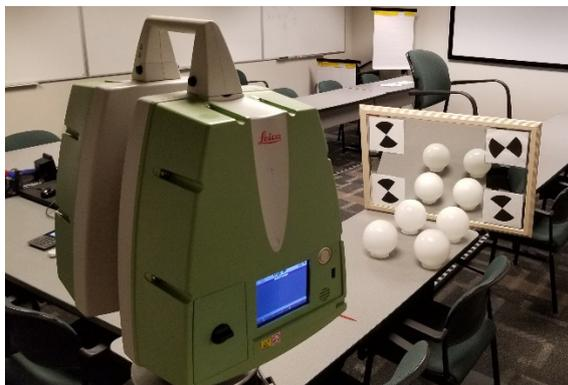
Figure 17: Experimental setup with P40 scanner.
