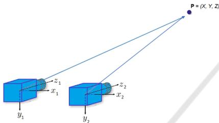
Figure 3: 3D point,  $P$ , observed by the same camera at two different poses.
