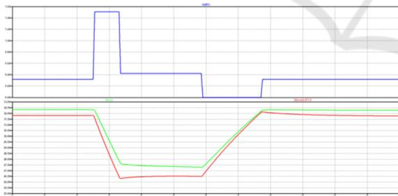
Figure 3: Example of simulating the temperature of skin exposed to a cold pulse thermal excitation. The upper waveform represents the TEC current vs. time. The lower curves show the temperature (1 V corresponds to 1°C) vs. time. The green curve shows the skin surface temperature at the contact zone. The red curve shows the temperature of the thermo-display (TEC) under the skin.
