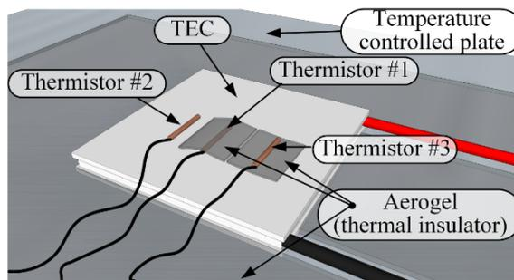
Figure 5: Scheme of experimental thermo-display and monitoring thermistors' layout.
