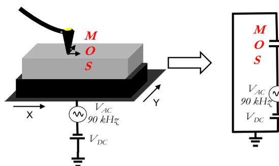
Figure 10: Scanning Capacitance measurement.
