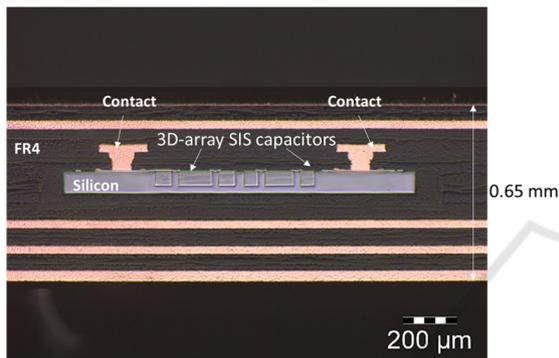
Figure 9: SIS capacitors embedded into a FR4 packaging.
