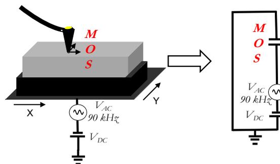
Figure 10: Scanning Capacitance measurement.
