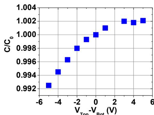
Figure 7: Capacitance variation of the SIS capacitor as a function of the applied voltage,  $C_0 = 25 \text{ nF/mm}^2$ .
