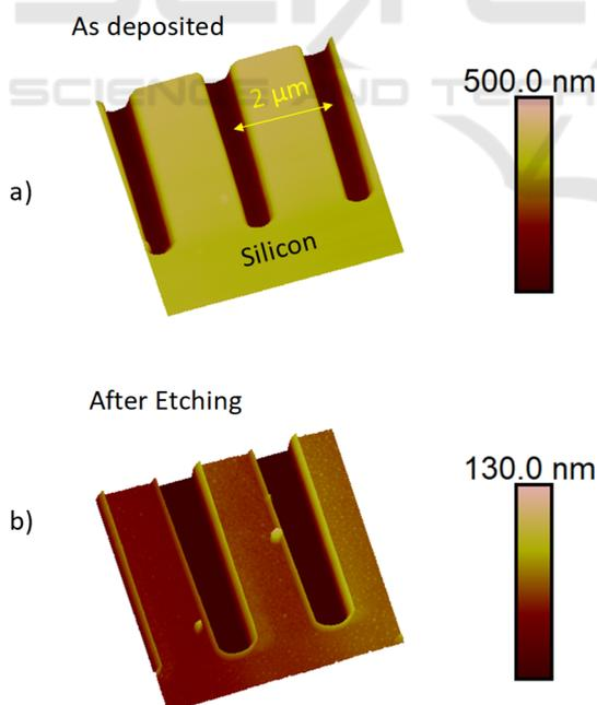
Figure 3: AFM topography measurements of the dielectric layers in the 3D structures  $5 \mu\text{m} \times 5 \mu\text{m}$ , a) as-prepared, b) after plasma etching to reveal the dielectric layer, before filling of the pores.
