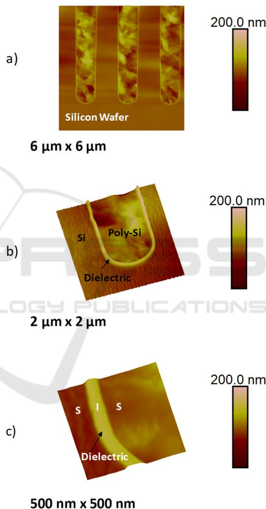
Figure 4: a) Scan of  $6 \mu\text{m} \times 6 \mu\text{m}$  of the bottom of the SIS capacitor after polysilicon filling, b) topography of  $2 \mu\text{m} \times 2 \mu\text{m}$  and c) zoom  $500 \text{ nm} \times 500 \text{ nm}$ .
