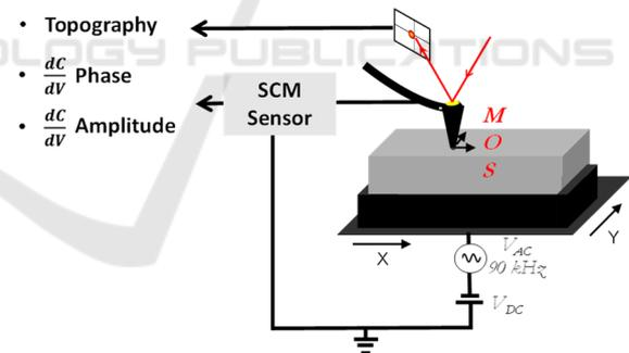
Figure 2: Schematic of the SCM mode based on an AFM, topography and local capacitance variation on the nano-MOS (the conductive tip in contact with the semiconductor) in phase and amplitude, simultaneously.
