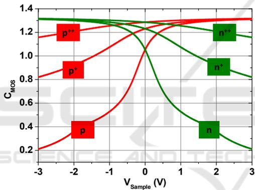
Figure 11: Optimization of SCM parameters, C-V calculated for various doping types and levels.
