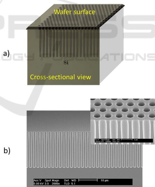
Figure 1: Silicon wafer after the etching of micropores inside the substrate, a) top-view and cross-sectional optical images of the wafer and b) cross-sectional SEM observations before filling.
