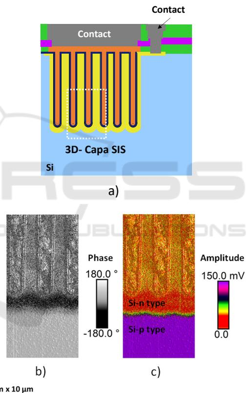
Figure 5: SCM results, scan size:  $5 \mu\text{m} \times 10 \mu\text{m}$  a) Schematics of the capacitor structure, with top and bottom electrodes on the same wafer side. b) SCM phase signal and c) SCM amplitude cartography of the area marked by a rectangle in a).
