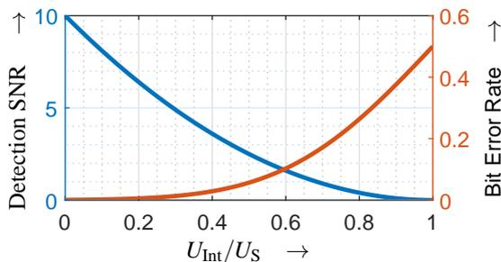
Figure 3: Relation between combined interferences  $U_{Int}$ , detection SNR  $\rho$  and bit error rate (BER)  $P_E$ , assuming  $P_N = 0.1 \text{ V}^2$  and  $U_S = 1 \text{ V}$ .
