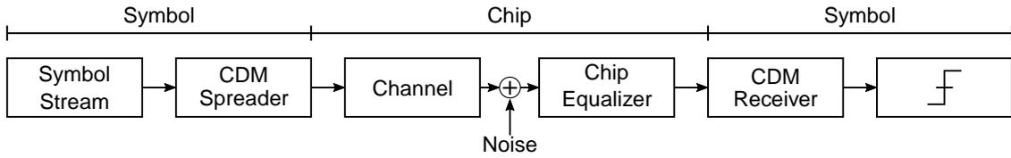
Figure 6: Simulation of data transmission using a single user CDM system.
