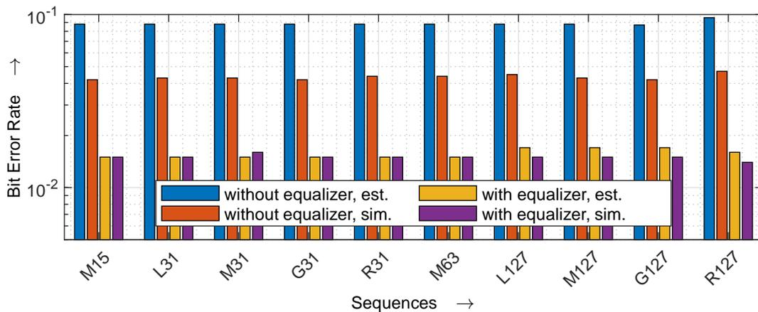
Figure 7: Simulated BER as a function of selected code sequences with an SNR  $10 \cdot \log_{10}(E_s/N_0)$  of 10 dB.
