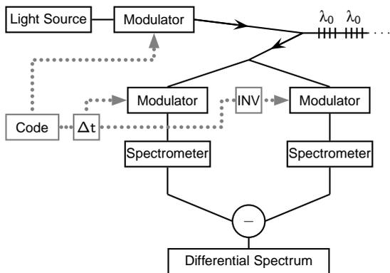
Figure 1: Setup of CDM Interrogation System (Götten et al., 2020).
