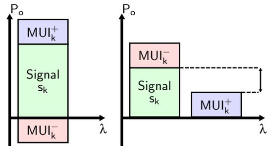
Figure 4: Graphic representation of mSMUI, where  $P_o$  is the spectral optical power density depending on the wavelength  $\lambda$ .
