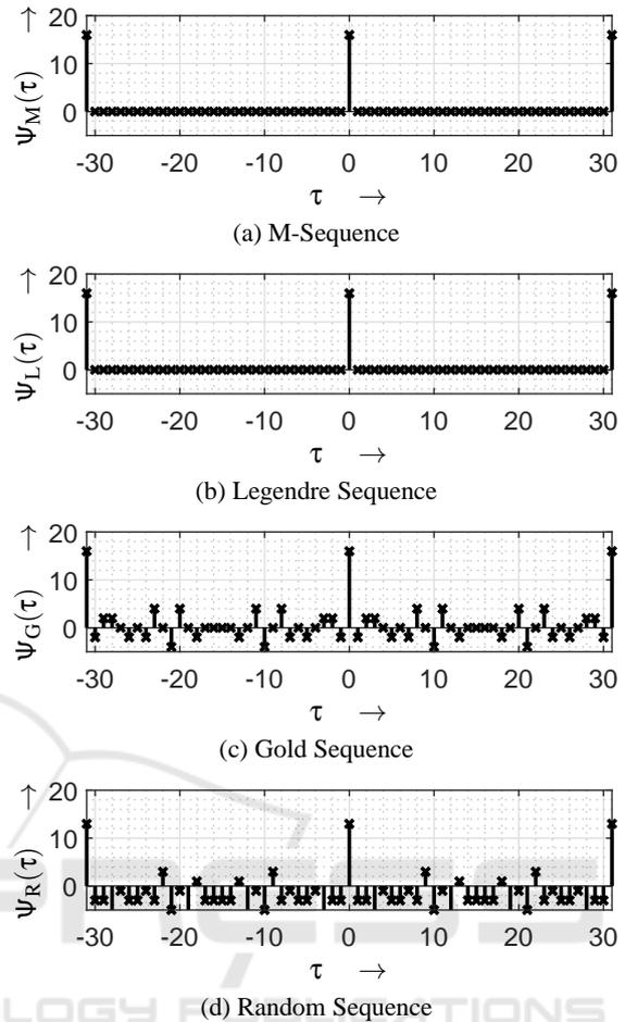
Figure 2: Cyclical autocorrelation function (ACF) obtained applying SIK of different sequence types with a length of 31 chips.
