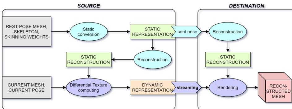
Figure 1: Overview diagram of our method for animation compression and reconstruction.
