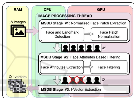
Figure 2: MSDB procedure in the image processing thread.
