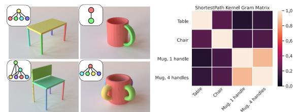
Figure 1: Objects are automatically segmented and part graphs are created. Shape descriptors of parts serve as node attributes in the graph. Relying on this, graph kernels can be used to estimate similarity of objects.
