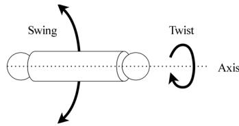
Figure 2: Left sphere is the parent joint and right sphere is the child joint. There is a limb between both joints. The joint rotation for the parent joint is decomposed into swing and twist rotations.
