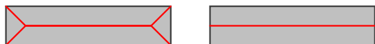
Figure 2: The result of a medial axis transformation (left) and the midsurface transformation of a thin-walled part (grey) are usually different. As the midsurface has to respect follow-up simulation usages, both results (left & right) may be a correct midsurface depending on the application context.
