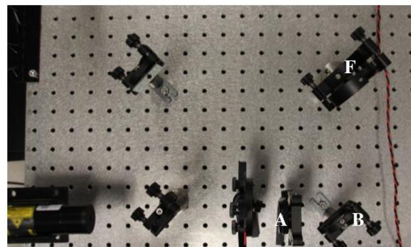
Figure 6: Mechanical setup for the proof of concept. (A) helium-neon laser at a wavelength of 632.8 nm, (B) beam splitter, (C) sample, (D) pinhole, (E) flat mirror, (F) flat mirror, (G) beamsplitter.
