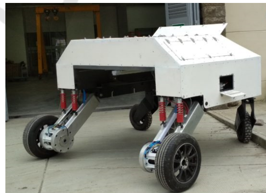
Figure 1: CERES robot: Agricultural robotic platform electrically powered with two brushless motors liquid-cooled (each motor is 5KW) attached to a gearbox 50:1 these are coupled to a car wheel of a common rin 14. CERES has a payload of 100 Kg of solid fertilizer, 20 liters for fumigating purposes and a weeding system. For the high-level processes, CERES uses a 9 DOF IMU, a LIDAR and stereo cameras are integrated.
