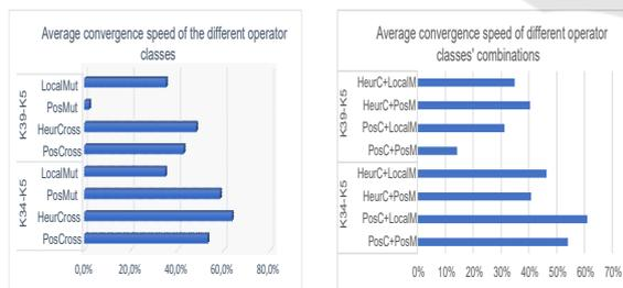
Figure 2: Convergence Speed according to the maximum number of iterations for each class or combination of classes of operators for the CVRP instance n34-K5 and n39-K5.
