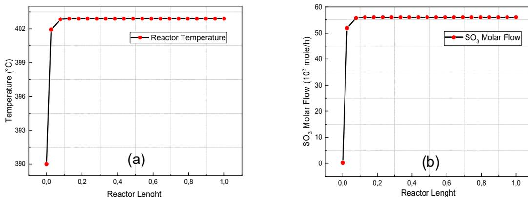
Figure 5: Temperature (a) and SO<sub>3</sub> molar flow (b) variations in the 4<sup>th</sup> catalytic bed.
