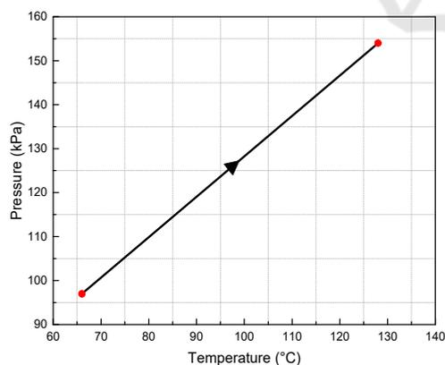
Figure 4: P-T curve of the air compressor.
