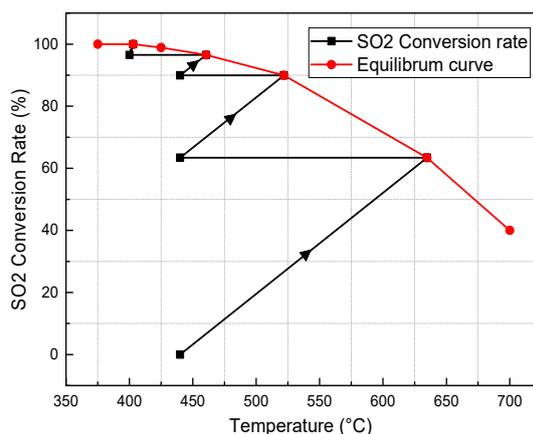
Figure 7: Conversion-Temperature curve of the catalytic converter.
