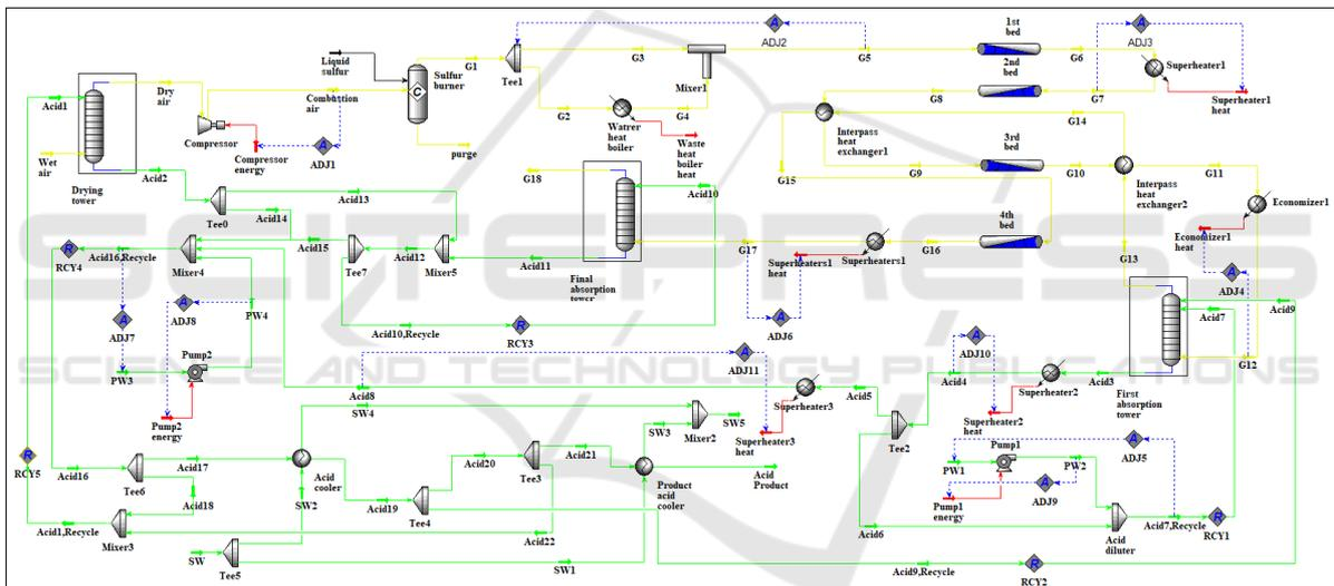
Figure 2: UniSim-Design simulation of the sulphuric acid manufacturing process with double absorption.
