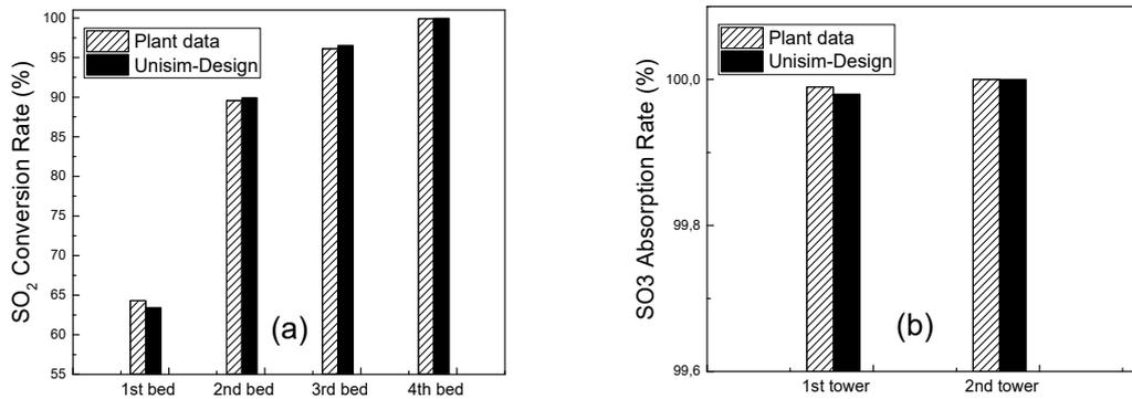
Figure 8: UniSim Design converter (a) and absorption towers (b) simulation results versus plant data.
