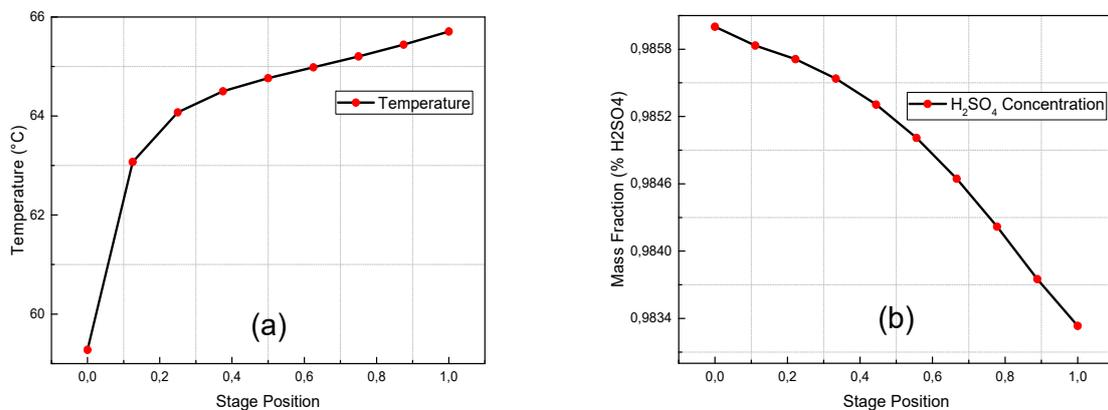
Figure 3: Temperature (a) and sulphuric acid concentration (b) variations in the drying tower stages.
