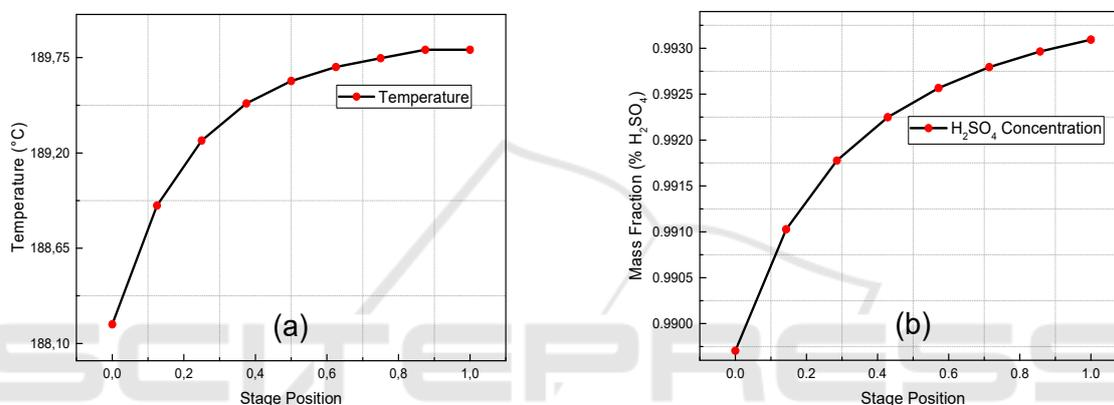
Figure 6: Temperature (a) and sulphuric acid concentration (b) variations in the first absorption tower.
