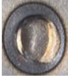
Figure 2: Poor-quality spot causes by misalignment.
