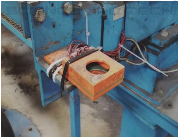
Figure 12: Actual PCB location for magnetic field measurement.
