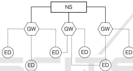
Figure 3: LoRaWAN architecture.
