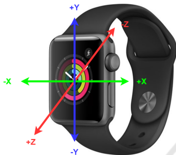
Figure 3: Apple watch series-1 used for recording accelerometer and gyroscope signals.
