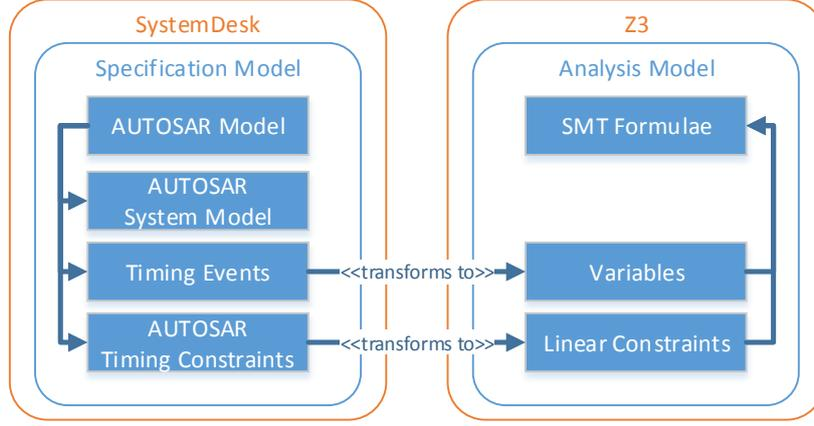
Figure 3: Transformation of AUTOSAR models into SMT formulae.
