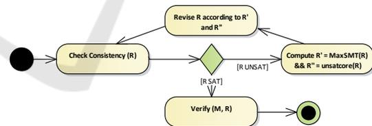
Figure 1: Analysis process described as UML activity diagram.
