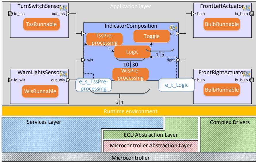
Figure 2: Example Software Architecture.
