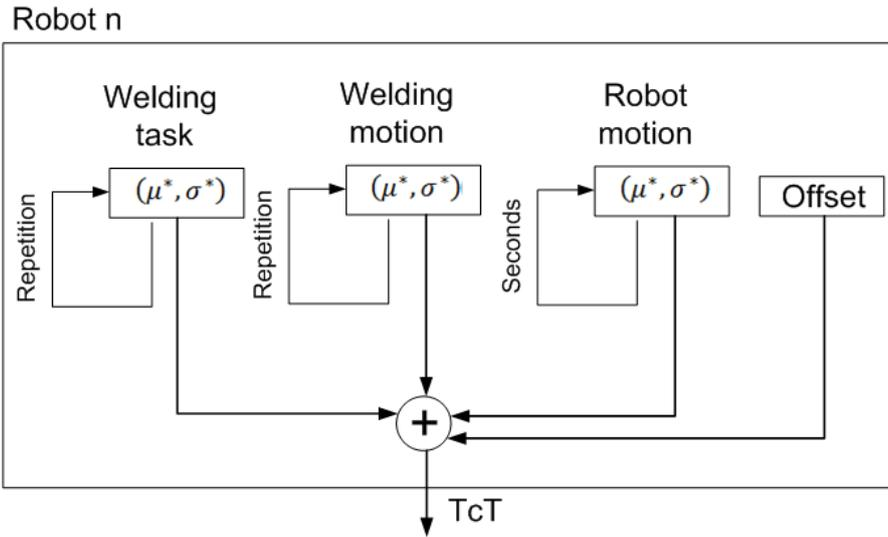
Figure 8: Cycle time computation for each robot/Welding unit.
