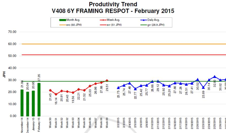
Figure 6: Jobs Per Hour produced in a real welding line VS idealized production rate. Note: ECR (engineering running capacity). ERR (engineering running rate). GRR (get ready requirement).
