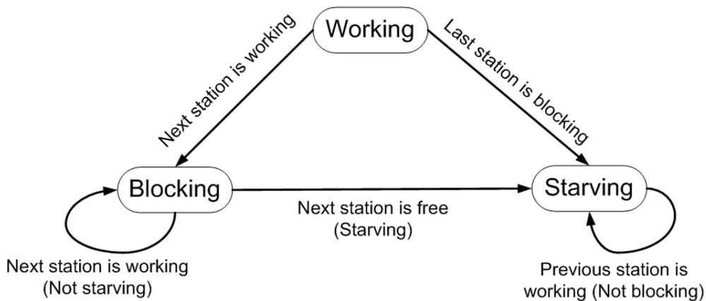
Figure 3: Simplified machine state for the workstation.
