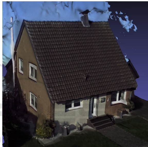
Figure 6: Resulting 3D model from Metashape (resolution 720p).
