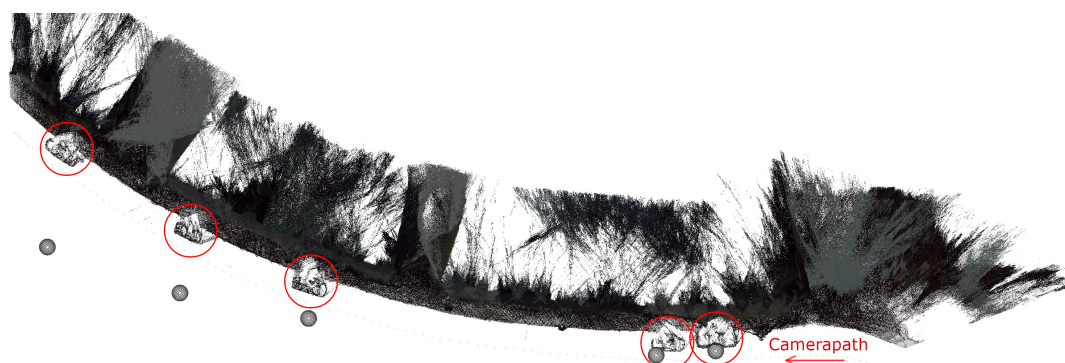
Figure 11: Imported standard objects at the detected positions of cars along a facade.
