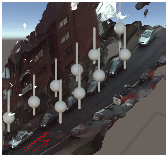
Figure 10: Imported standard objects at the detected positions of cars along a street.
