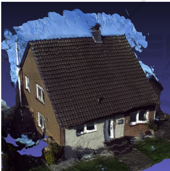
Figure 8: Resulting 3D model from Metashape (resolution 2.2K).
