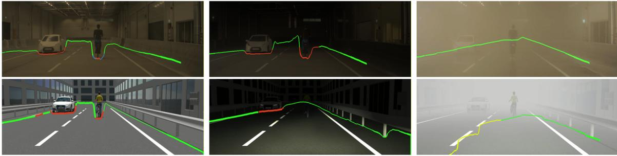
Figure 9: Real (top) and simulation-based (bottom) test drives with predictions of the free-space detection under different environment conditions: daytime (left), night time (middle) and fog (right). The free-space boundary lines display vehicles and bicycle in *red*; persons in *blue*; curb in *green* and others in *yellow*.
