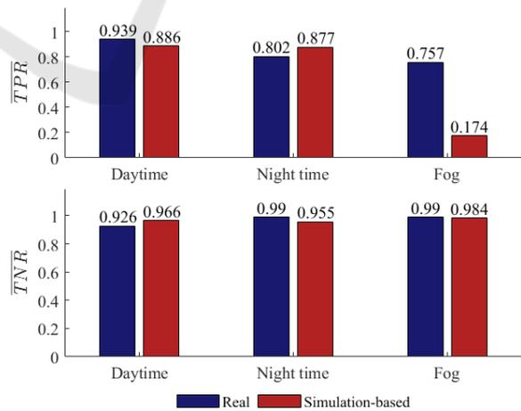
Figure 8:  $\overline{TPR}$  and  $\overline{TNR}$  results of the free-space detection under daytime, night time and fog conditions on real and simulation-based test drives.
