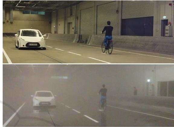
Figure 4: Inner-City test scenario built on the proving ground - daytime (top) and fog (bottom).
