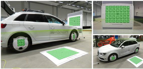
Figure 3: Camera calibration.
