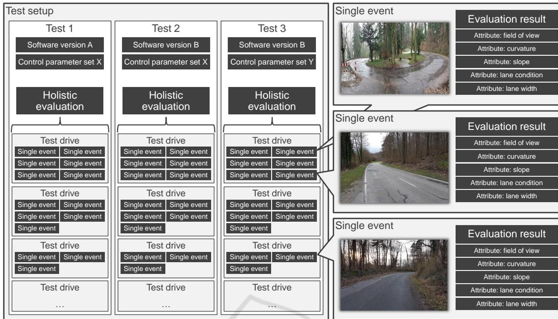
Figure 5: Test Setup with Different Software Versions and Control Parameter Sets Simulated with the Same Test Drives. Each Test Drive Has a Number of Relevant Events, Which Are Individually Evaluated. However, a Holistic Evaluation for Each Test Run Is Required to Compare the Tests.
