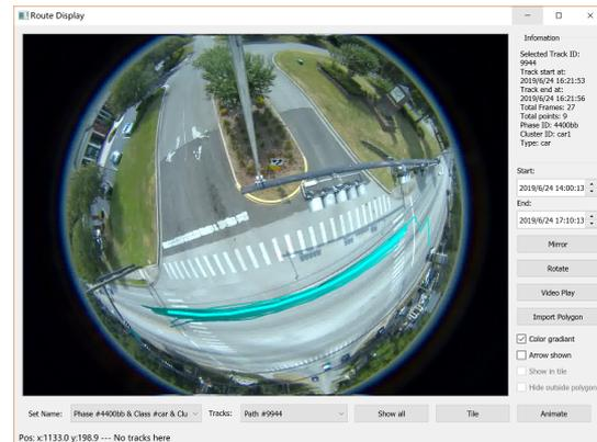
Figure 10: A specific track is selected among a set of tracks in Route Display. Information about the selected track appears on the right-hand side panel.
