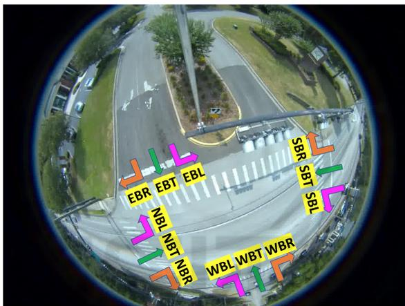
Figure 18: Representation of codes for allowed movements of vehicles at the intersection.
