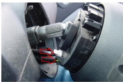
Figure 7: Steering angle sensor.
