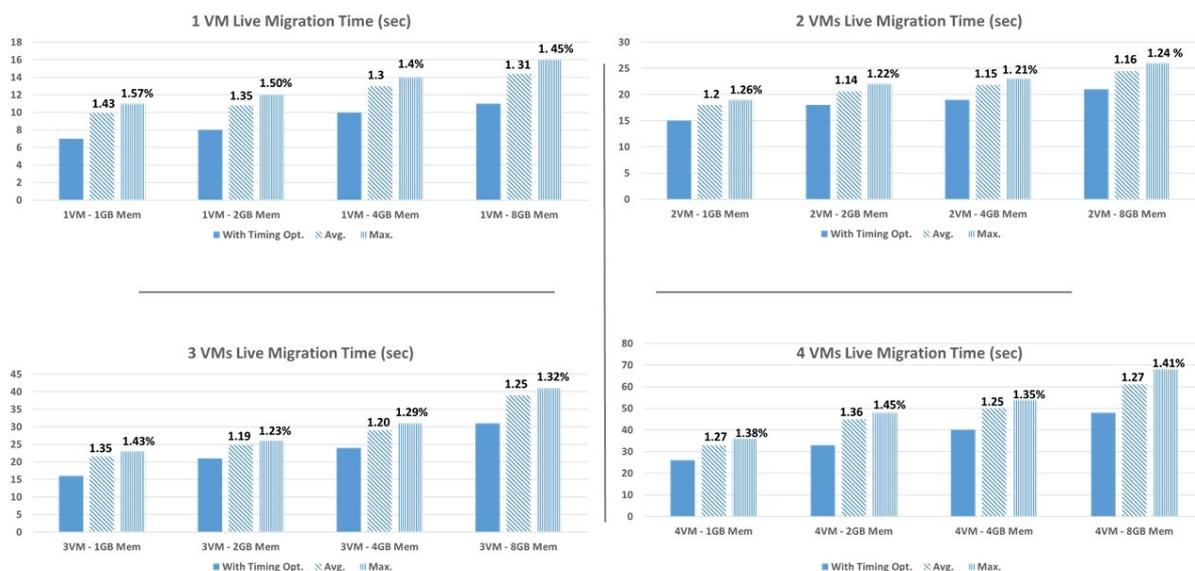
Figure 7: Network Stress - Impact of Timing Optimization on Live Migration Time.
