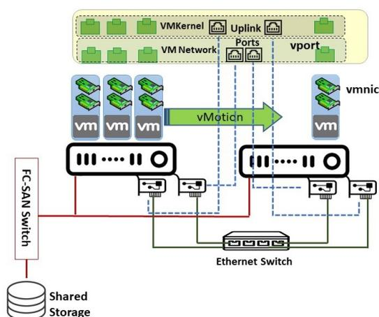
Figure 2: Network Topology for VMware vMotion.
