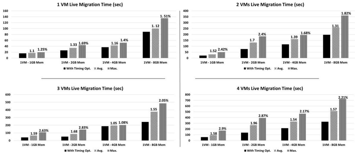
Figure 6: Memory Stress - Impact of Timing Optimization on Live Migration Time.
