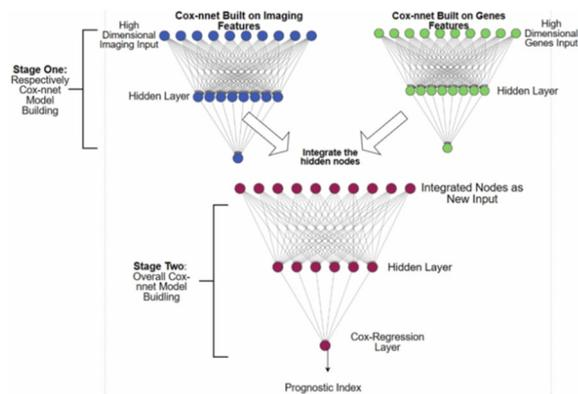
Figure 5: The architectures of 2-stage Cox-nnet complex model for prognosis prediction, which integrates multiple data types (eg. pathology image and gene expression).
