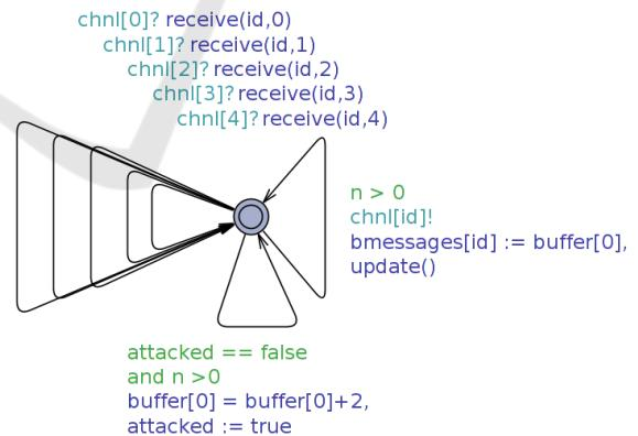
Figure 9: Template modeling the tamper attack.
