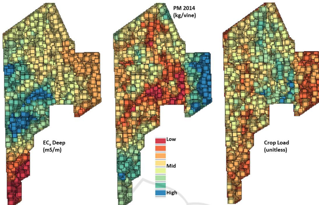
Figure 6: Images Illustrating the Spatial Patterns of the Three Input Variables - Apparent Soil Electrical Conductivity (Left,  $EC_a$ ) to a Depth of 1.5 M Using a Dualem 1s (DUALEM, Mississauga, ON, Canada); Pruning Mass (Centre, PM 2014) from 2014 Predicted from a Calibrated Canopy Sensor ((Taylor et al., 2017) and Crop Load (Ravaz Index) in 2014 Using the Pruning Mass and Grape Yield Monitoring Data (Yield Data Not Shown).
