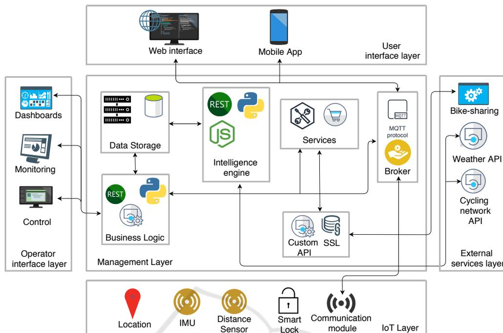
Figure 2: Connectivity Platform Architecture.
