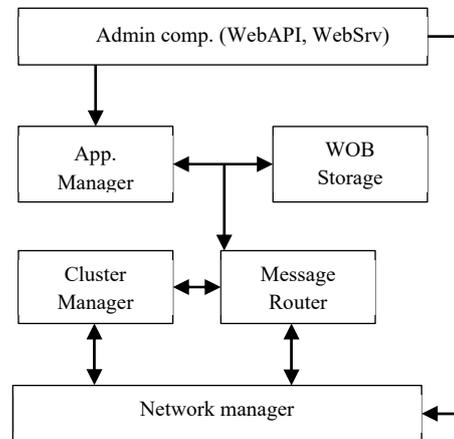
Figure 3: Middleware internal structure.
