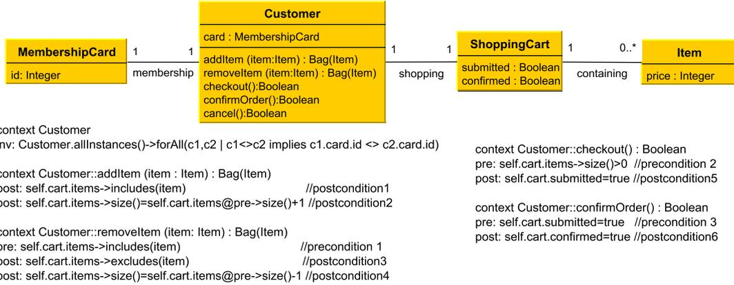
Figure 1: A UML class diagram annotated with a set of OCL operational contracts models an online shopping system. *inv* here specifies a class invariant. *pre* and *post* specify preconditions and postconditions of an operation respectively. @pre here denotes an object from previous state.
