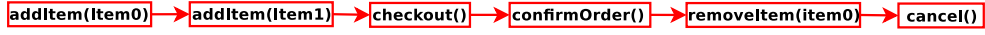
Figure 2: A call sequence shows a scenario that a customer may modify items after confirming an order.
