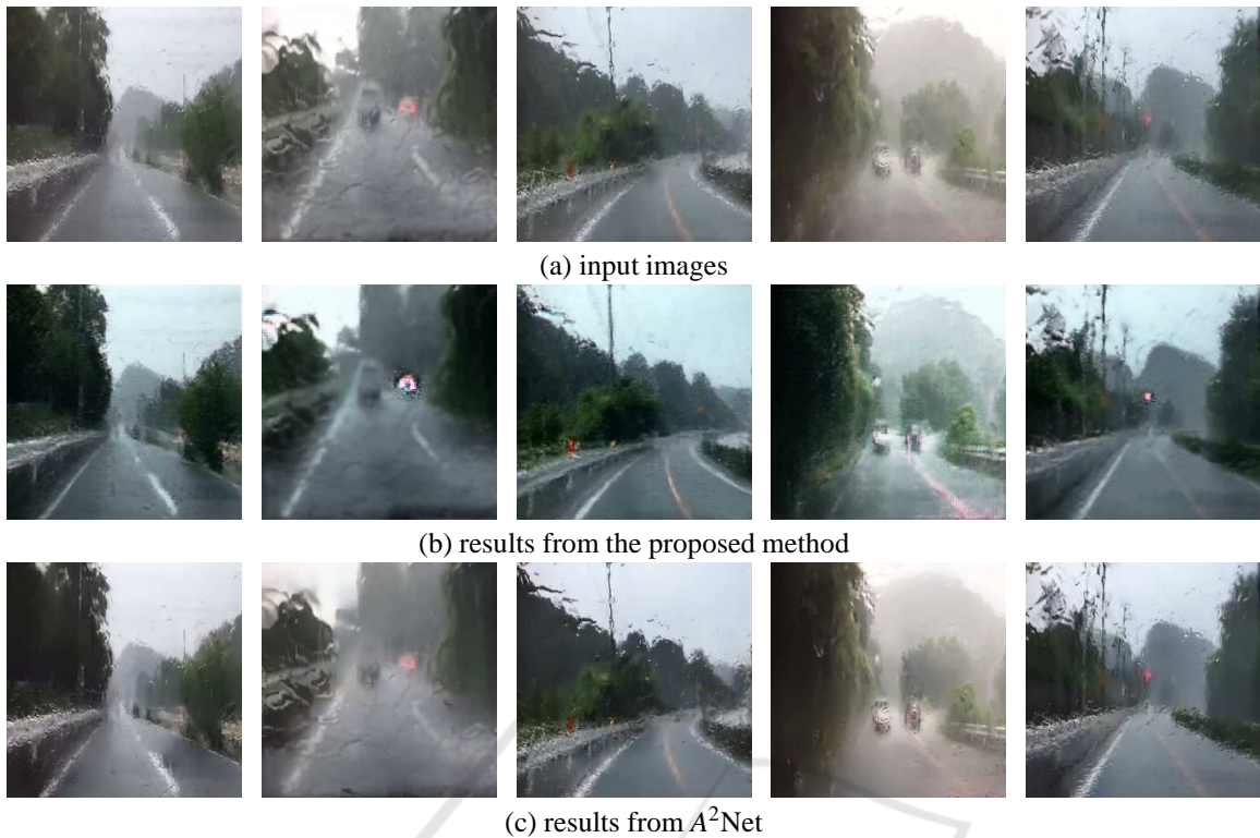
Figure 11: Results from real image experiment. (a) shows images observed under heavy rain. (b) and (c) show raindrop removal images obtained from images in (a) by using the proposed method and A^2Net respectively. The visibility in (b) is better than that in (a) and (c). For example, the white lane markers and the road guardrails are heavily distorted in (a) and (c), but they look more accurate in (b).
