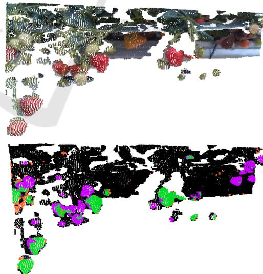
Figure 4: The segmentation results for  $PNet_{colour}$  trained on data from the stereo camera: the original point cloud (top), segmentation results (bottom). The colours indicate: TP in green, FP in orange, FN in purple and TN in black.
