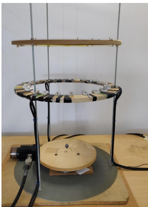
Figure 2: A picture of the laboratory-developed US imaging system. Sensors (1 Tx, 21 Rx) are located on a wooden ring. The multiview-multistatic configuration is realised via a rotating table the targets are located on, in order to virtually simulate the movement of the sensors ring.
