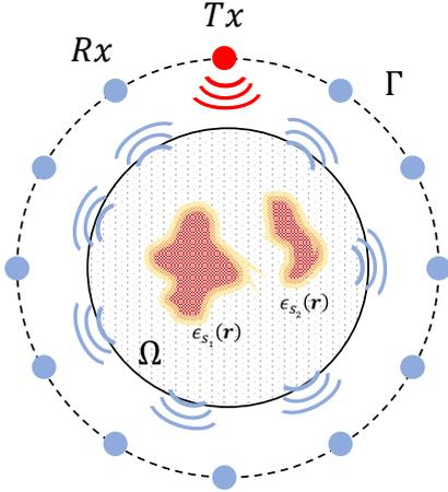
Figure 1: Sketch of the multiview-multistatic imaging system for the non-invasive testing of the imaging domain  $\Omega$ . The antennas are located on a measurement curve  $\Gamma$ .
