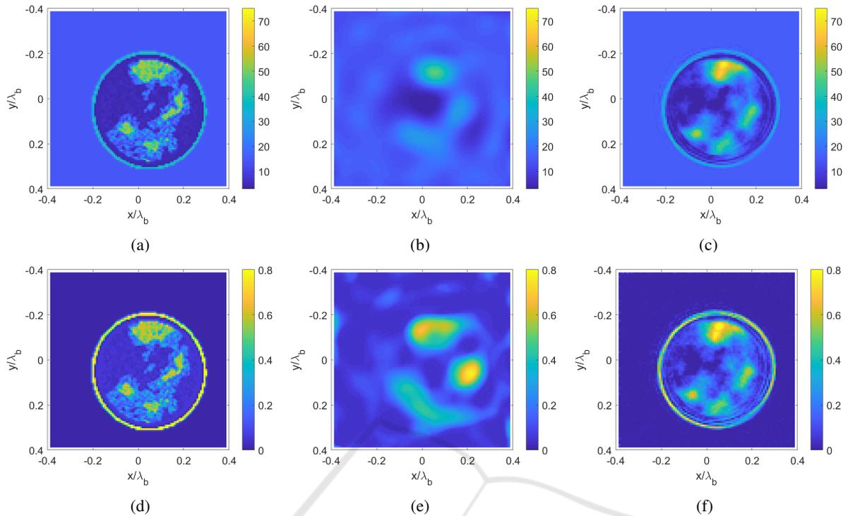
Figure 3: Numerical results (a),(d) real and imaginary parts of the reference complex permittivity, respectively; (b),(e): retrieved profiles via a classical non-linear approach (distorted-Born iterative method) and (c),(f) via the proposed neural network architecture.
