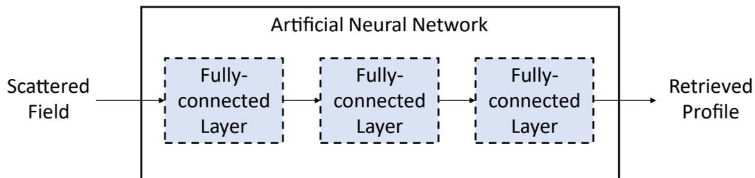
Figure 2: Architecture of the proposed network. This direct inversion scheme has the samples of the scattered field as input and provides an estimate of unknown complex permittivity profile maps as output.
