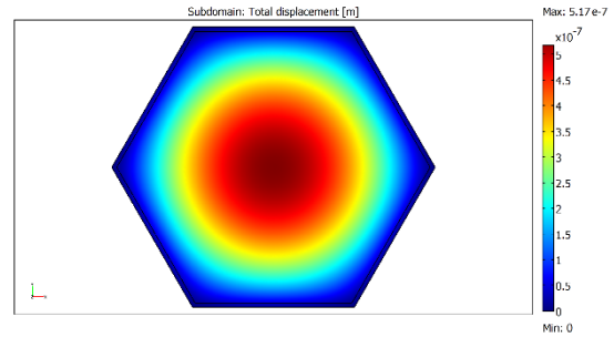
Figure 1: Simulation result of mirror plate deformation with FEM in COMSOL.
