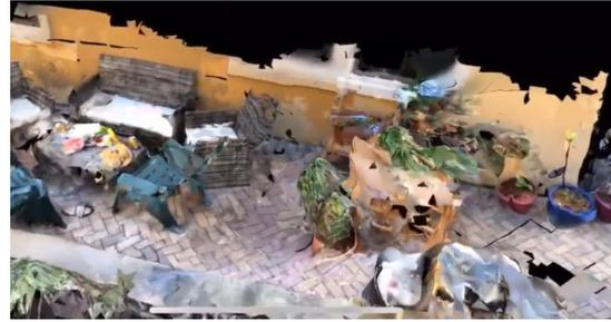
Figure 7: Realtime generated 3D mesh of local scene captured from a smartphone.
