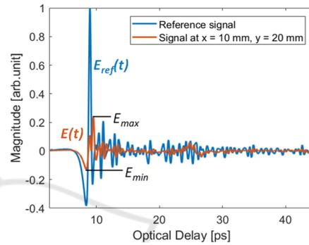
Figure 4: Example of a recorded IR of the sample, in red, and the recorded reference IR (using a gold-coated alignment mirror), in blue.
