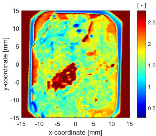
Figure 8: THz FD image of absorbance at 1 THz, as defined by Eq. (4).
