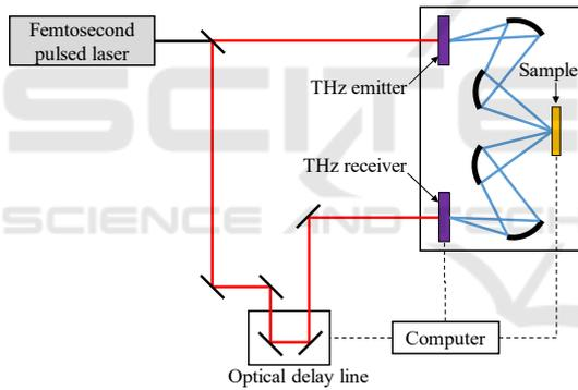
Figure 2: Schematic diagram of the experimental setup used to measure the reflection THz IR of the sample.
