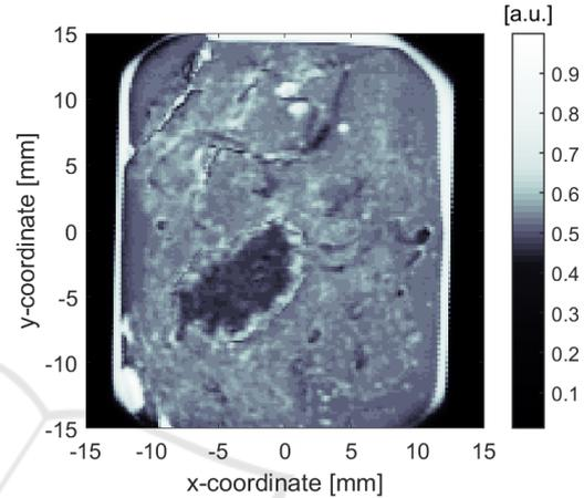
Figure 6: THz TD image obtained using the normalized peak-to-peak amplitude of the IR, as defined by Eq. (2).
