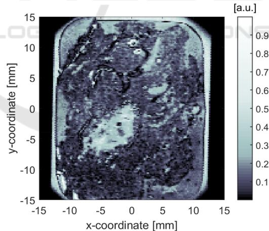
Figure 7: THz FD image obtained using the normalized magnitude of the FR at 2.5 THz, as defined by Eq. (3).
