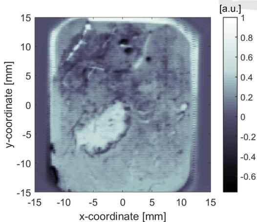
Figure 5: THz TD image obtained using the normalized amplitude of the IR at optical delay  $t_d$  of 9 ps, as defined by Eq. (1).
