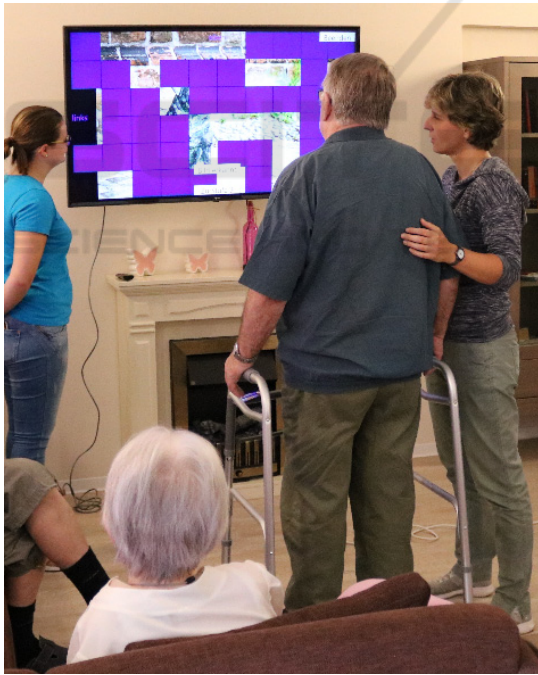
Figure 1: Setting of the training sessions. The elderly stands on the force plate, which is surrounded with a safety construction. A coach, nurse or caregiver supervised the elderly during the training. During playing the elderly sees the changes made by moving the center of gravity on the screen and step-by-step the hidden image becomes visible.
