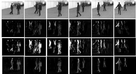
Figure 3: First-row: original video frames of moving people; second-row: extracted foregrounds with standard DMD method; Third-row: extracted foregrounds with compressed DMD; Last-row: extracted foregrounds with dl-DMD (Proposed).
