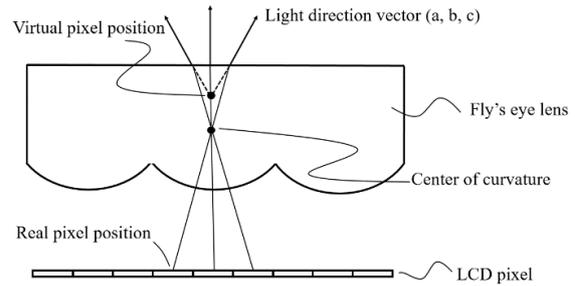
Figure 3: Path of light emitted from LCD pixels.
