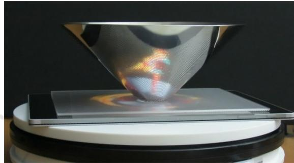
Figure 11: Autostereoscopic image displayed with our system on an electric turntable (© UTJ/UCL).
