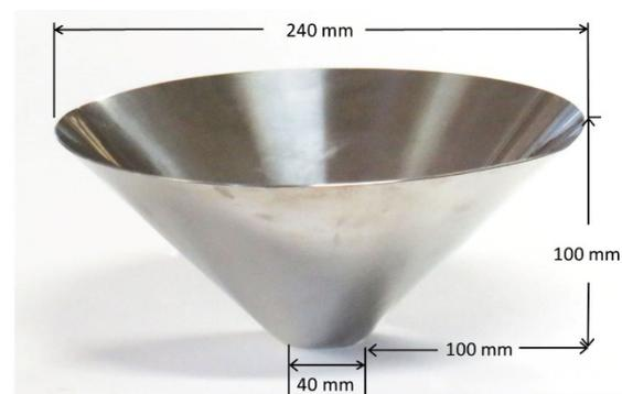
Figure 8: Conical mirror.
