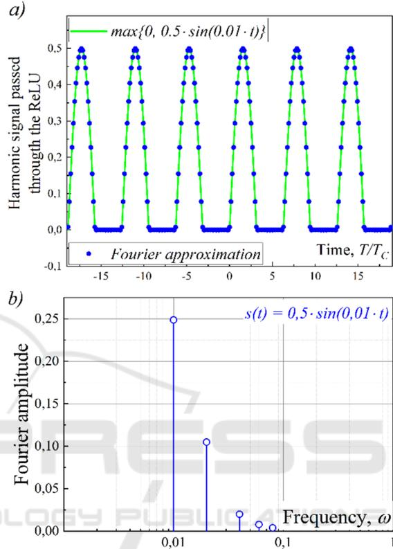
Figure 3: The result of passing through a mathematical ReLU a simple harmonic signal and its approximation using the Fourier series (a) and the Fourier spectrum of the output signal (b).
