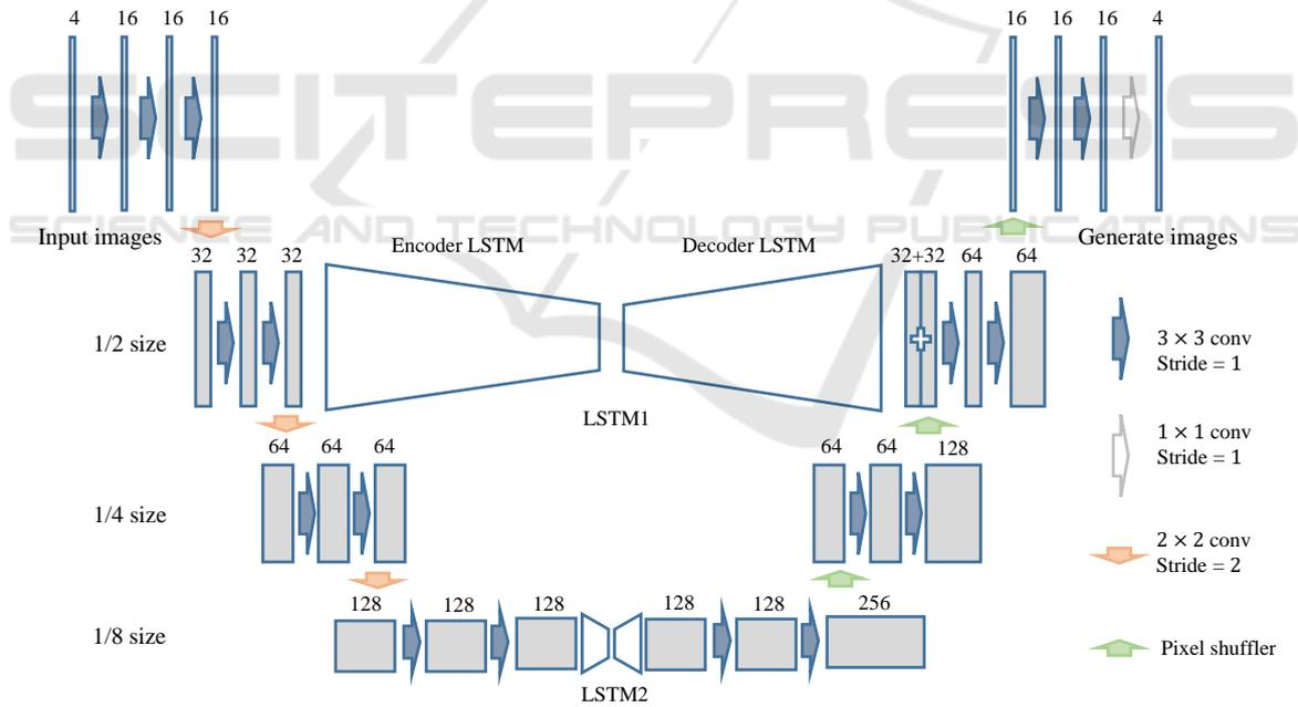
Figure 2: Generator. Each image is spatially convoluted through the CNN, and transformed with time information through the LSTM. The converted image is restored by CNN and pixel shuffler.
