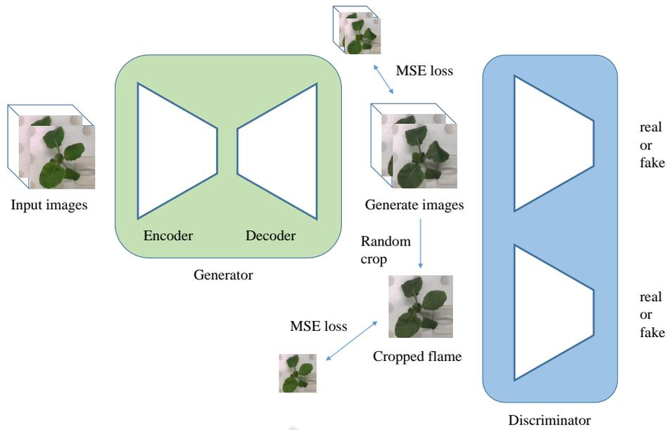
Figure 1: Proposed network for 3D plant growth prediction. The network converts the RGB-D plant image input through the generator into a predicted one several hours later. In the GAN process, the generated image is discriminated from the correct image by discriminator.
