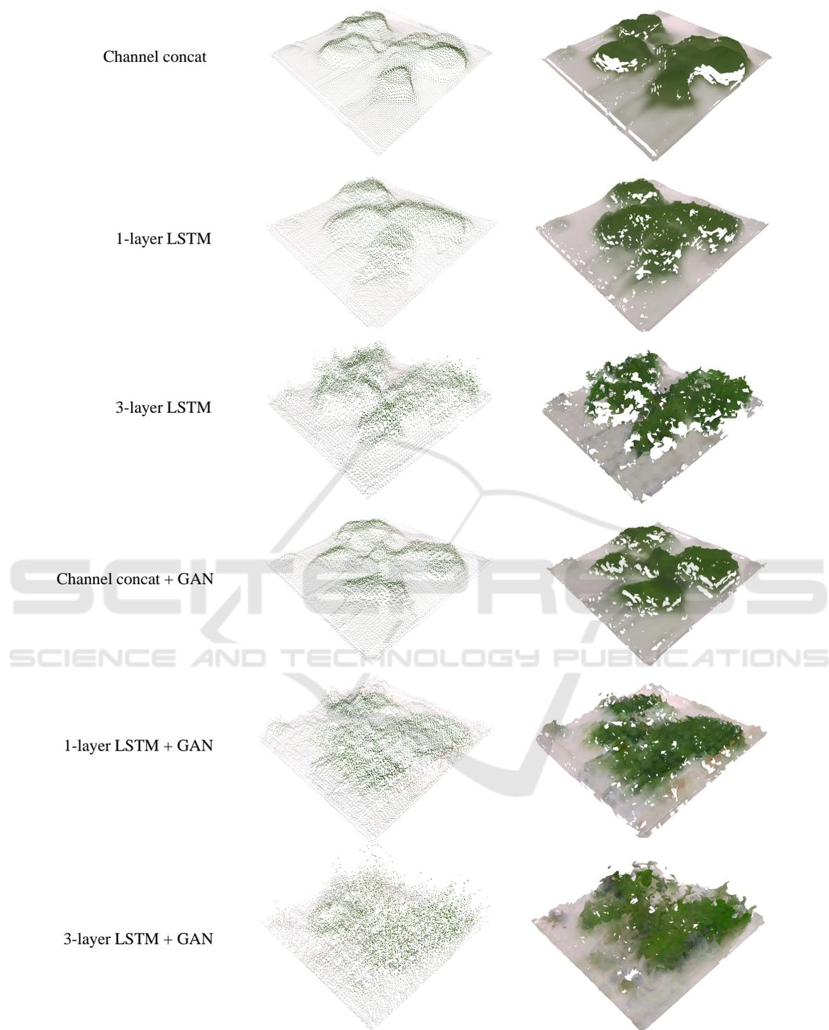
Figure 8: 3D restoration result of predicted image. 3D point cloud (left) and faceted image by Ball Pivoting (right) are visualized.
