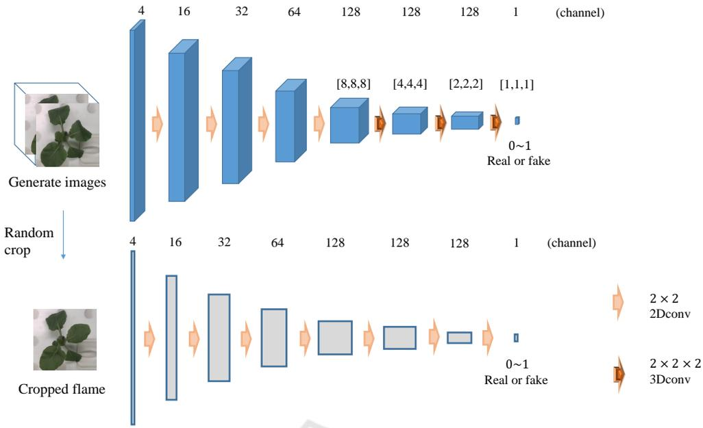
Figure 4: Discriminator. The discriminator has a single image identification function and a time-series image identification function. 3D convolution is used for the time-series image discrimination.
