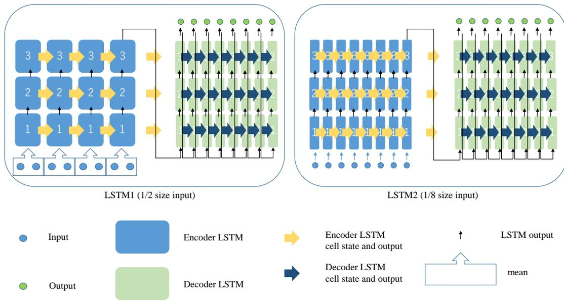
Figure 6: 3-layer encoder-decoder LSTM. The LSTM output is passed to the next LSTM. The output of the last layer of the decoder LSTM is regarded as the output of the entire encoder-decoder.
