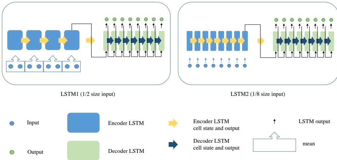
Figure 3: Encoder-decoder LSTM. The encoder of LSTM1 has an input that averages two elements of 1/2 size of the original image, and LSTM2 takes 1/8 element of the original image as input. The decoder receives the output and cell state of the final layer of the encoder.
